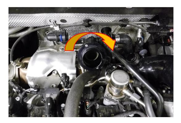
10. Push the Forge vacuum T over the vacuum port on the inlet manifold, secure it with the E-clip provided and reconnect the OEM vacuum hose (removed in Step 2.) to the other side of the Forge vacuum T.
