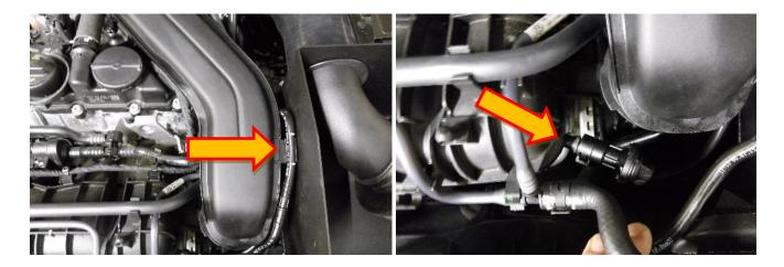
3. At the end of the boost inlet pipe nearest the back of the engine, turn the twist fit coupler anti clockwise to unlock it and un-clip the Norma fitting on the breather pipe.
