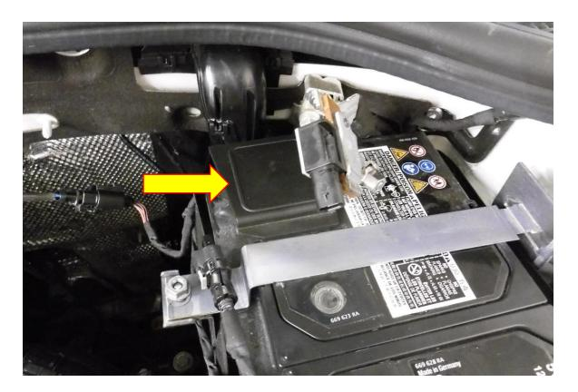
2. Using a 10 & 13mm socket and ratchet remove both fasteners attaching the clamps to the battery. You will now be able to remove the battery from the vehicle.
