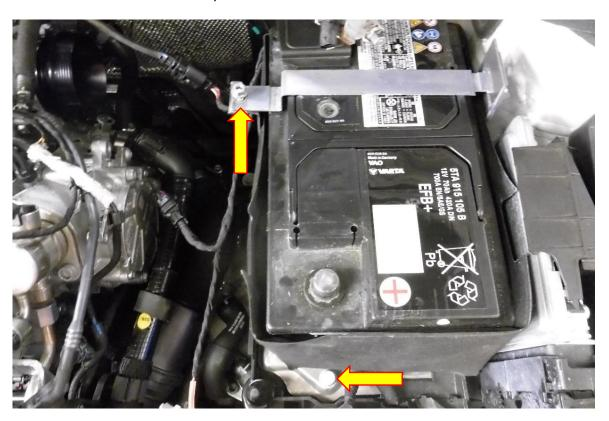
3. Using a 13mm socket and ratchet remove the fastener attaching the bracket to the battery tray. Remove the bracket and turn 180 degrees then re fit and fix it back into place. Now re install the battery.
