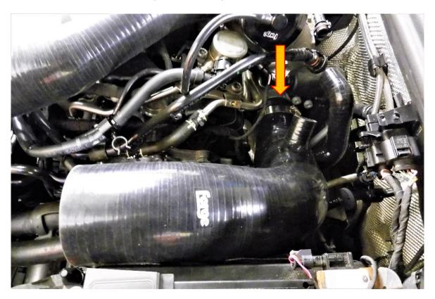
10. Take the breather adaptor and insert the billet end into the spout coming from the Forge intake hose. Secure it in place with the supplied 16-27 hose clamp, then re fit both breathers. If you are not installing our recirculation valve (FMDV30) install the supplied alloy blanking plug and secure it with the other 16-27 hose clamp.
